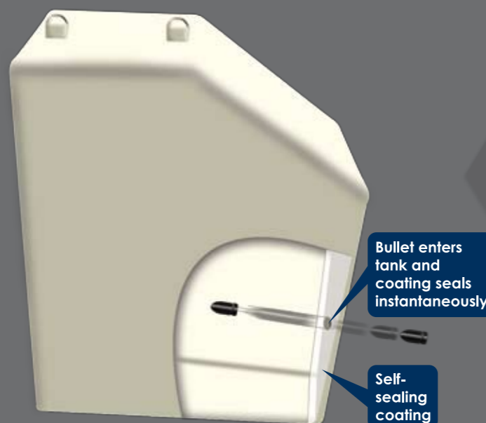
Cross-section of fuel tank
