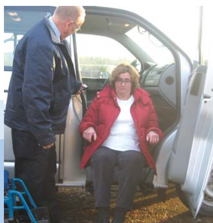
VW Transporter T5 with Turny installed on the front passenger seat.
