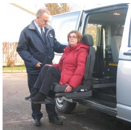
Turny Orbit is easy to handle. The driver just pushes a button to ease the passenger into the vehicle. Here is the product installed on the right-hand side of the central row in a VW Transporter T5.
