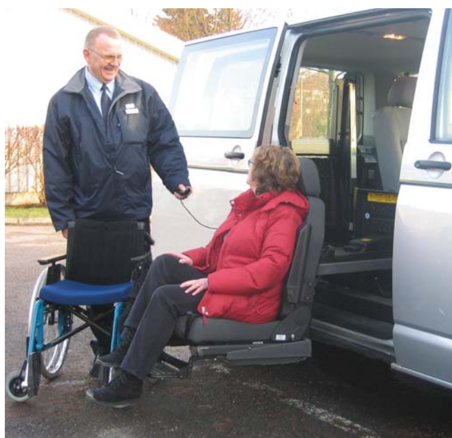
Turny Orbit is easy to handle. The driver just pushes a button to ease the passenger into the vehicle. Here is the product installed on the right-hand side of the central row in a VW Transporter T5.
