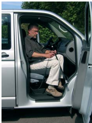
2. Press the button on the manual control to swivel the seat outwards.
