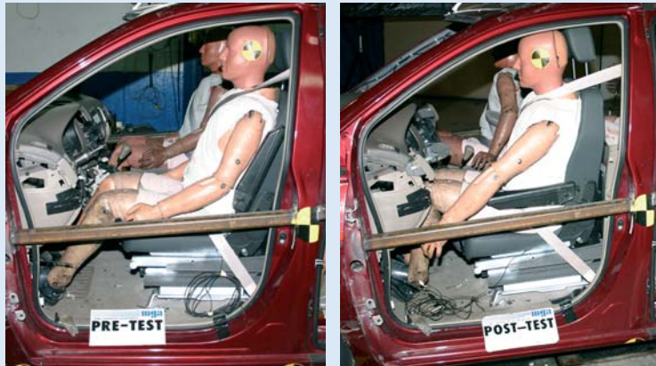
Crash test of a Turny Orbit in a Toyota Sienna.
