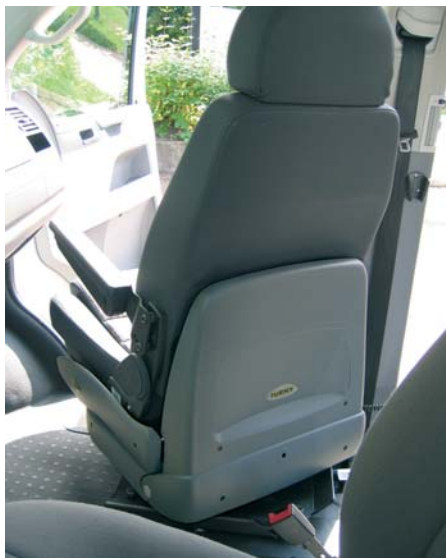
Turny HD fitted with the BEV-seat (an optional extra).
