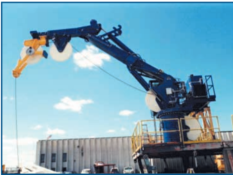
In-plant testing of a self-contained electro-hydraulic towing crane with electro-mechanical cable on a U.S. Navy oceanographic vessel. A telescoping section is incorporated into the jib boom.
