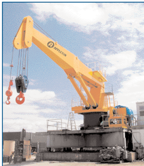
Appleton Marine's crane test platform can test cranes rated up to 10 million ft-lbs overturning moment and 15° list.
