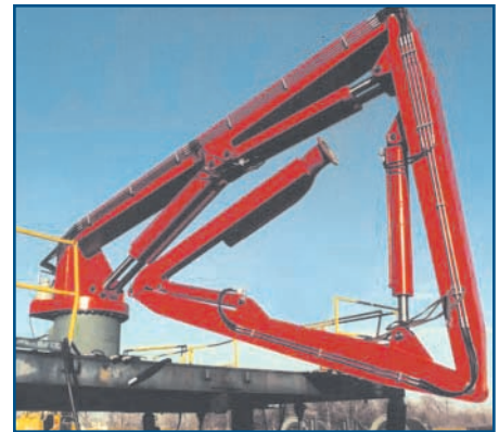
Articulated Boom Crane for handling pneumatic evacuation system for dry bulk materials
