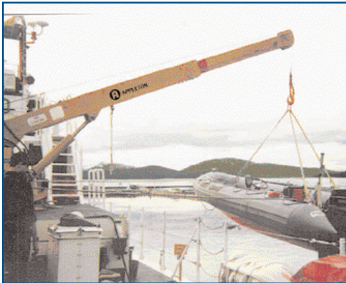
RHIB Handling Crane on USCG patrol boat
