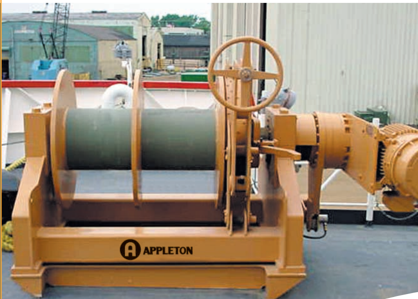
Powered Mooring System for USCG Great Lakes Ice Breaker
