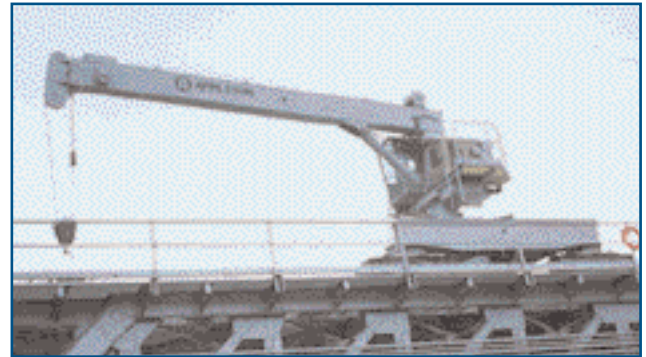
Army Corp of Engineers Lock and Dam Maintenance Crane
